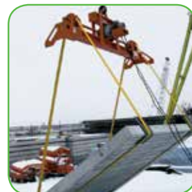
Load Rotating Beam
