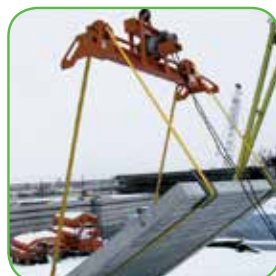
Load Rotating Beam
