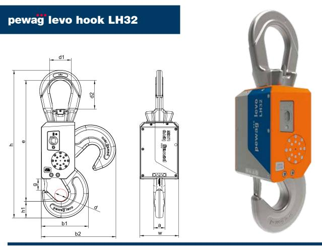
The pewag **levo hook LH32** comes with an additional brake that prevents the hook from automatically lowering when the hook is open. The optional magnet enables lifting of ferromagnetic materials weighing up to 12.5 kg. Furthermore, the placement of the magnet allows for effortless central positioning of the load.
