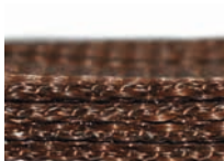
Webbing sling 4-layer structure
