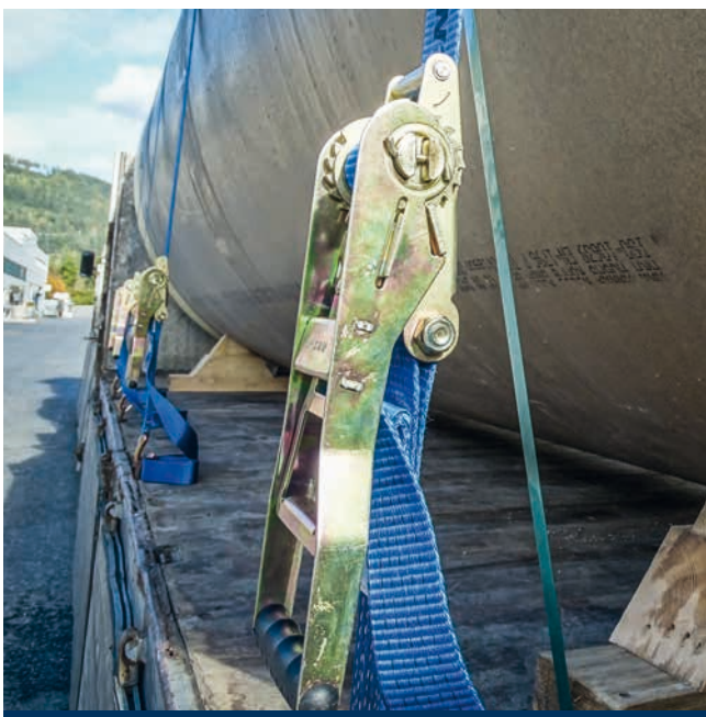
Long lever ERGO ratchet for higher standard tension force
