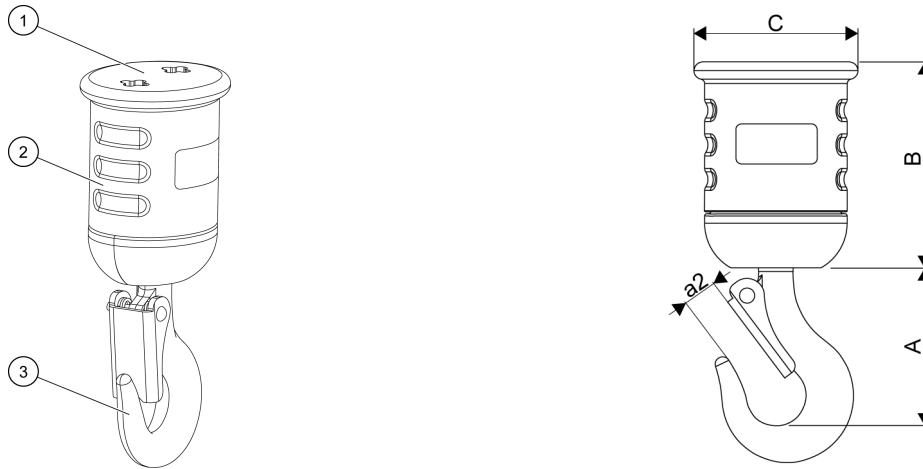
Figure 28. Two-fall (2/1) hook block for frame sizes 02–05
