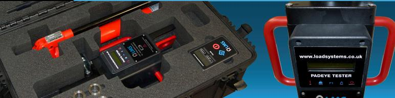
Lightweight, portable tool for testing pad eyes, lifting lugs, and eye bolts. It can be used upright, inverted, or in a horizontal plane. Models are available up to 50 ton proof test capability. Equipped with an adjustable clevis height and large dial capacity readout. Aluminum housing on 10 Te, 20 Te, and 30 Te models.
