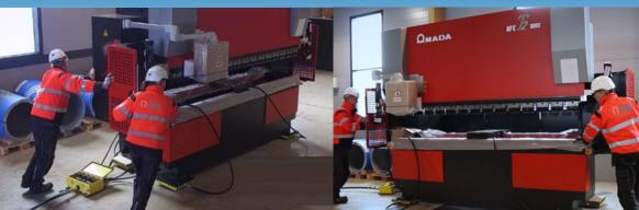
Air skates are robust, low profile, high capacity load-moving modules used in sets of four or more to enable large or heavy objects to be moved with ease.
